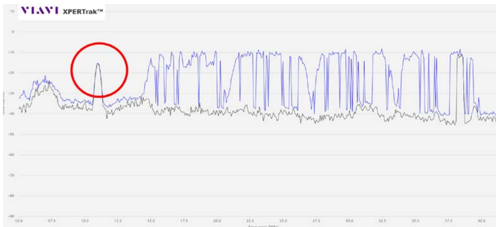
Figure 3 – Ingress shown in VIAVI XPERTrak span 5-42MHz
